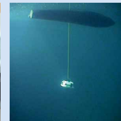
Model aero- and hydrodynamic tests in support of the design of the propulsion and control system of a mini-submarine
