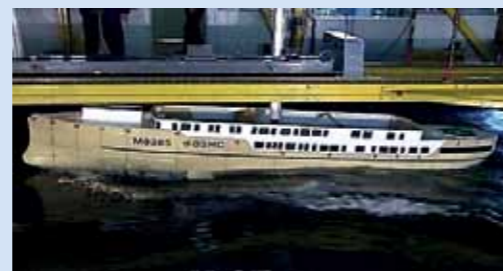
Optimization of the hull and the roll stabilization system of a mega-yacht using computer simulations and model tests at BSHC
