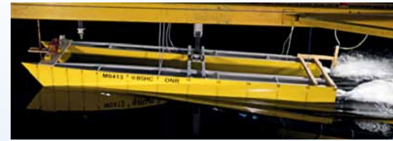
Numerical and physical modeling of a catamaran with water jet
