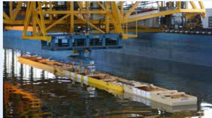
Model tests of a pusher and a push train at various water depths and various engine revolutions
