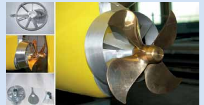
Ship model with Becker Mewis Duct® ready for towing tank testing
