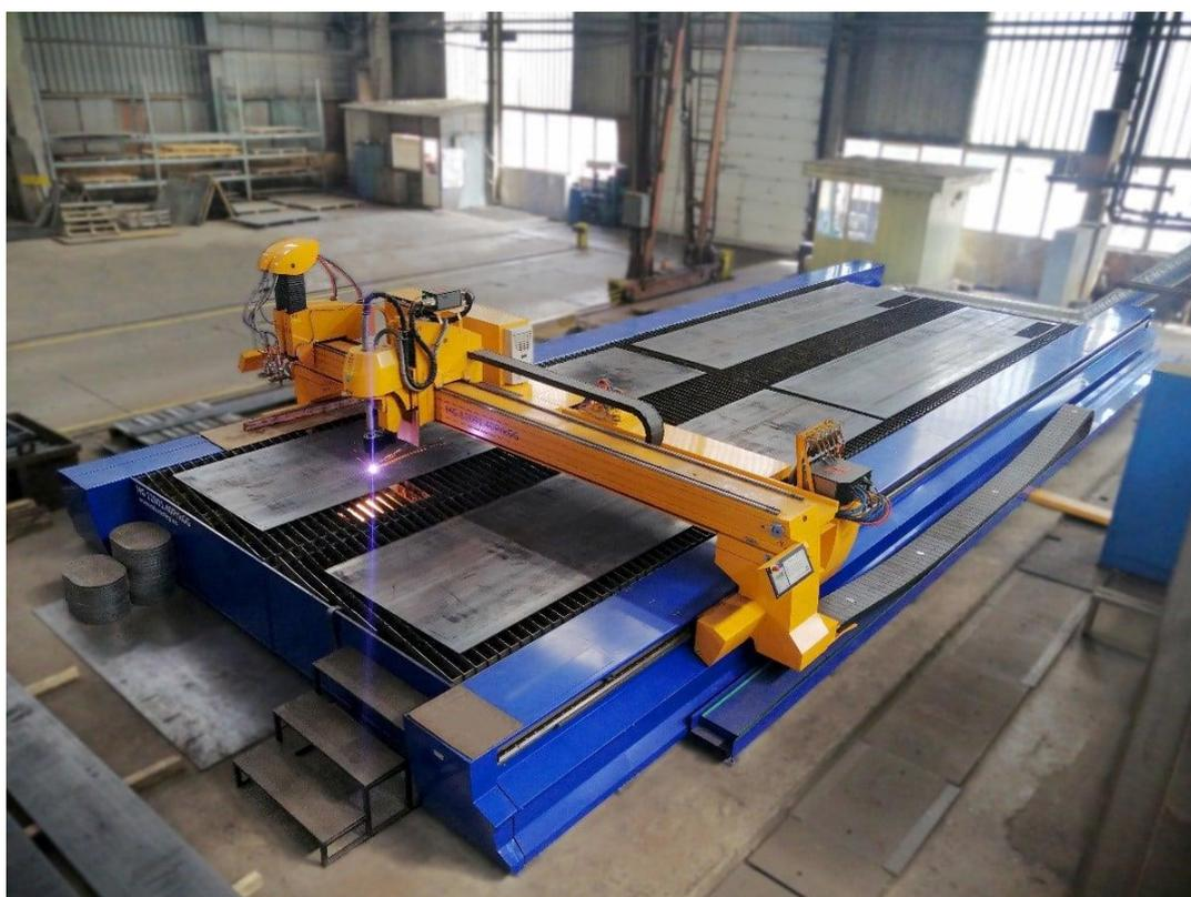
During this year TM Technology continued to invest in equipment, again on special order, buying bending machine for smaller details and new generation 6kW fiber optic laser with working area 2000x6000mm and maximum cutting thickness of metals up to 25mm.
