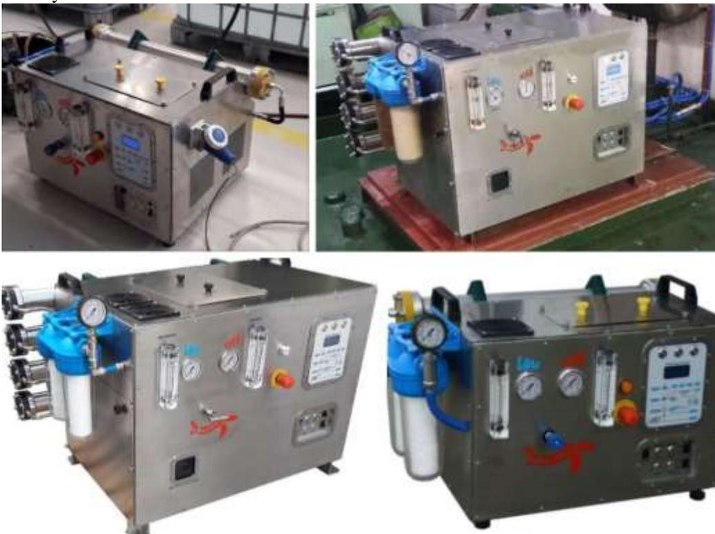
Taking into consideration that the reverse osmosis units do not require additional heat output (such as standard evaporators), they are flexible solution for water generation of the vessels with low power consumption.
