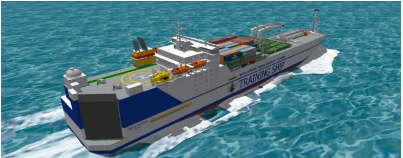
The ship is planned to be diesel - an electric power to make it more environmentally friendly and cost effective. Four diesel generators with a capacity of 14,400 kW (19,300 hp) Wärtsilä 12V46F each are provided to provide the necessary power supply. The propulsion system will be built from two 20,000 (27,000 hp) aspirators each and one WTT-55 WTT-55 5.5 kW (7.400 hp) turbocharger, which should provide very good maneuverability and maximum ship speed of 16 - 20 knots.
