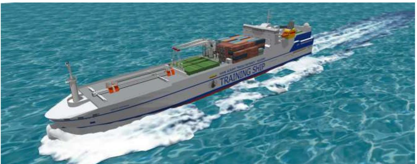
The car transport section is planned to be 200 - 300 carriages and will be located on four decks. Loading and unloading will be done by a hydraulic loading ramp in the stern of the ship.
