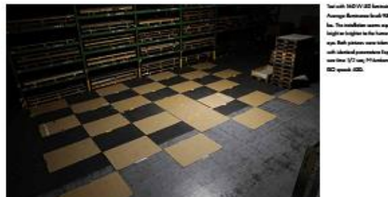
Test with 160 W LED luminaires. Average illuminance level: 95 lux.
