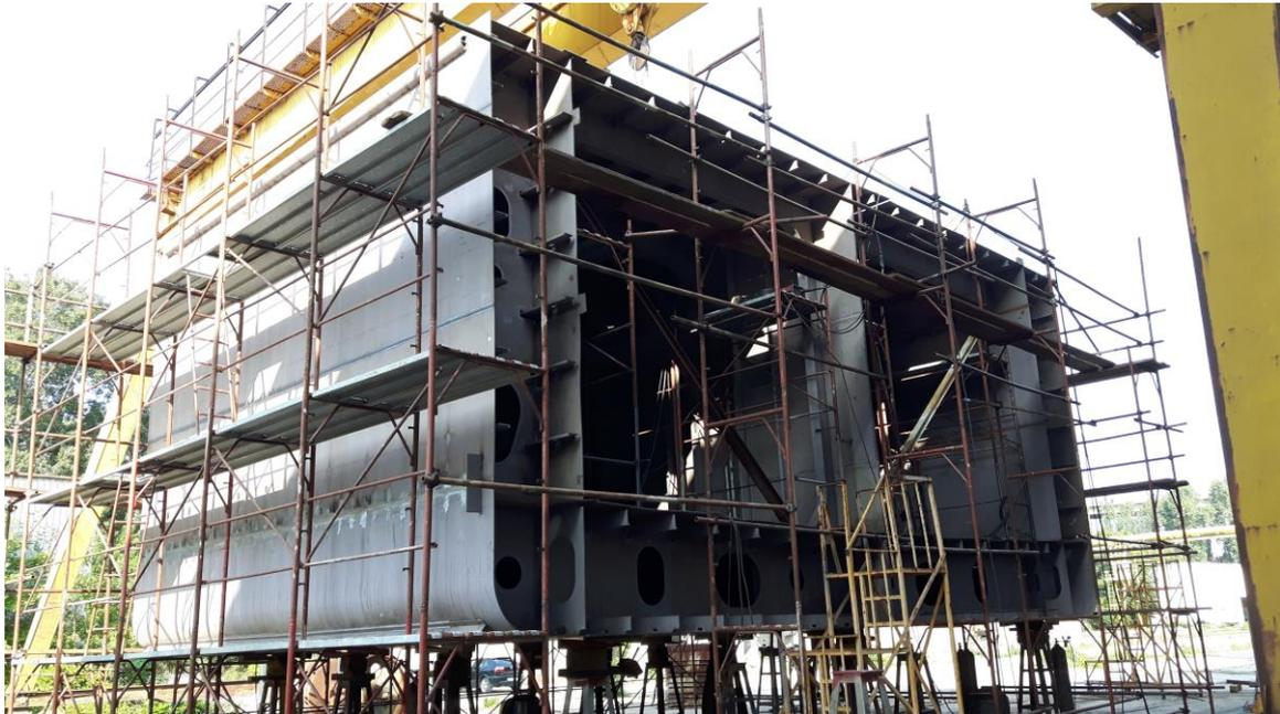
In June a new contract with TTS Marine AB was signed - for the manufacture of shipsets of panels for four ships under conversion. Each shipset weighs about 25 tons and consists of two couples of panels. The panels have unit dimensions of 15\*3,8 m. and are hinged in couples. The delivery of the first shipset is scheduled for September, and the remaining three will be delivered in November 2017.
